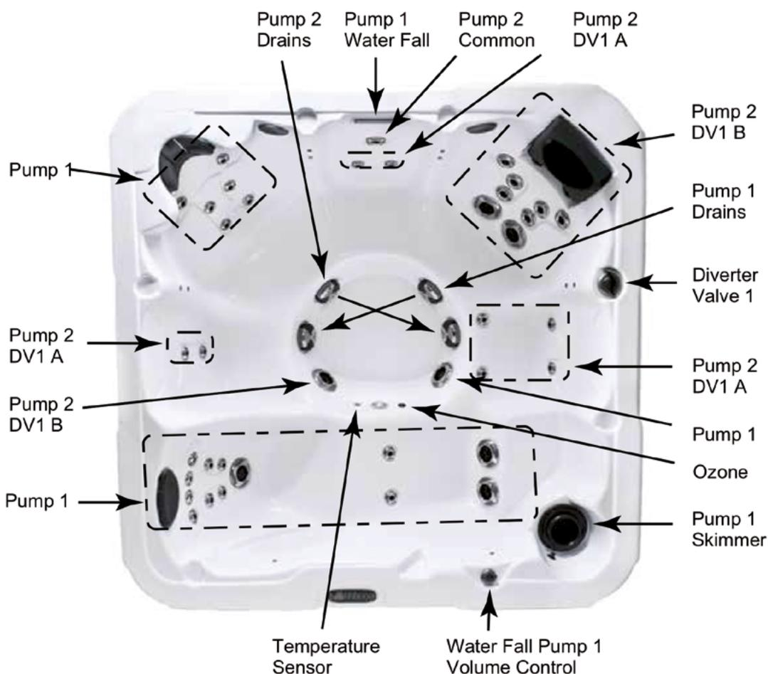
DV1 A = Diverter Valve 1 (A Position Clockwise)
